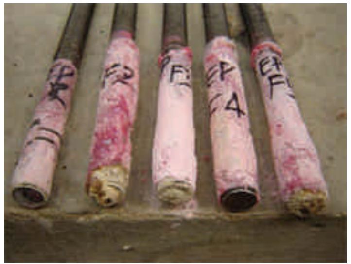
Figure 8.14: - Pull-out failure of Test No. EP20-F1 after tensile loading in wet unclean holes
