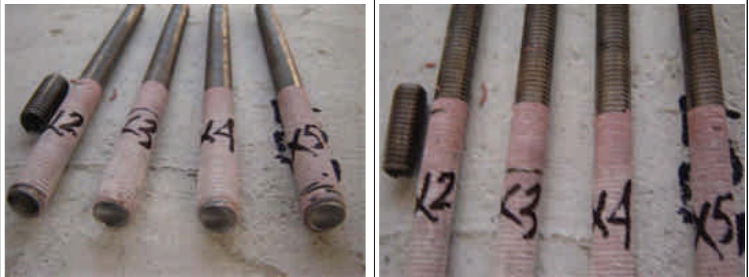
Figure 8.11: - Pull-out failure of Test No. EX12-A1 after tensile loading in dry cleaned holes
