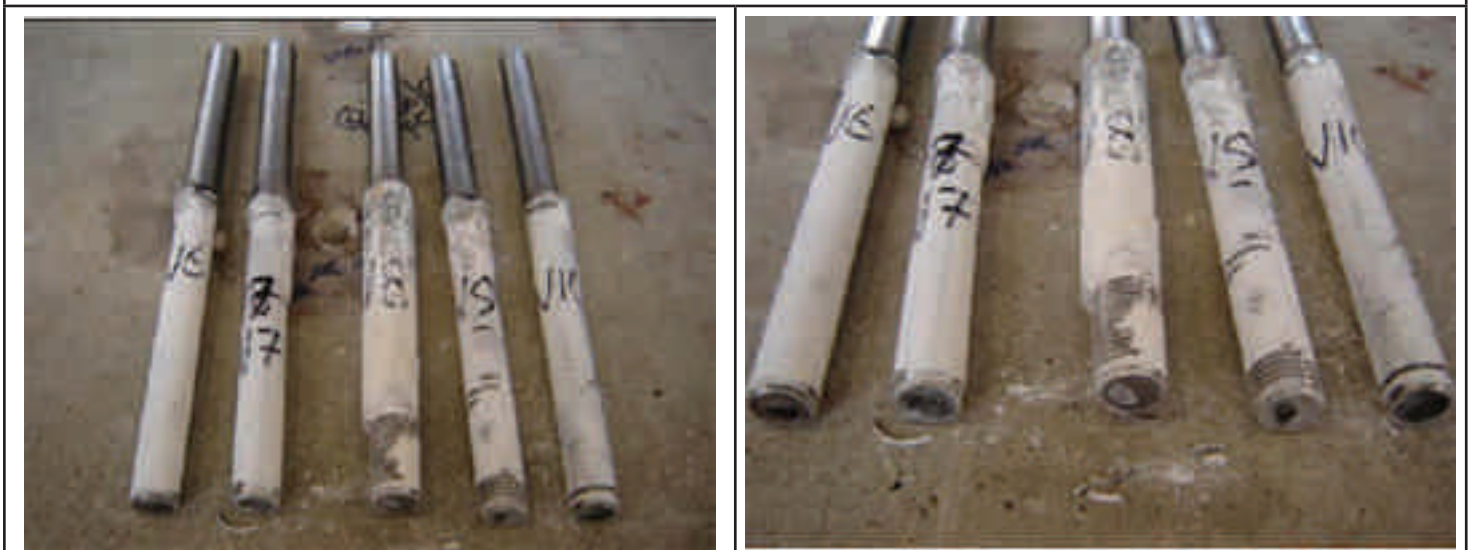
Figure 8.6: - Pull-out failure of Test No. VF20-A1 after tensile loading in dry cleaned holes
