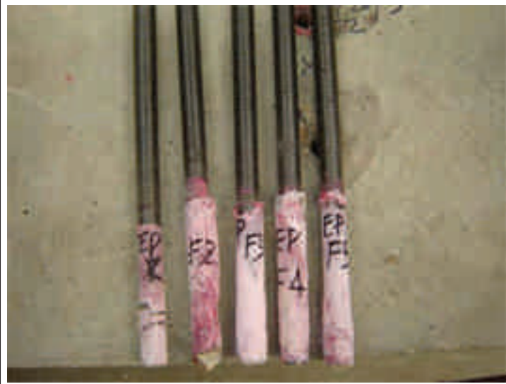
Figure 8.14: - Pull-out failure of Test No. EP20-F1 after tensile loading in wet unclean holes
