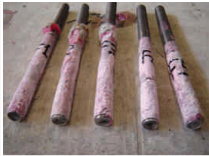
Figure 8.13: Pull-out failure of Test No. EP12-F1 after tensile loading in wet unclean holes
