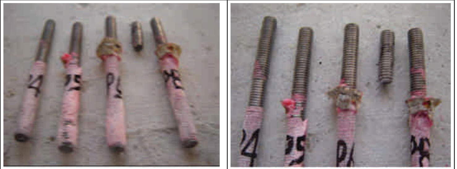
Figure 8.8A: - Pull-out failure of Test No. EP12-A1 after tensile loading in dry cleaned holes
