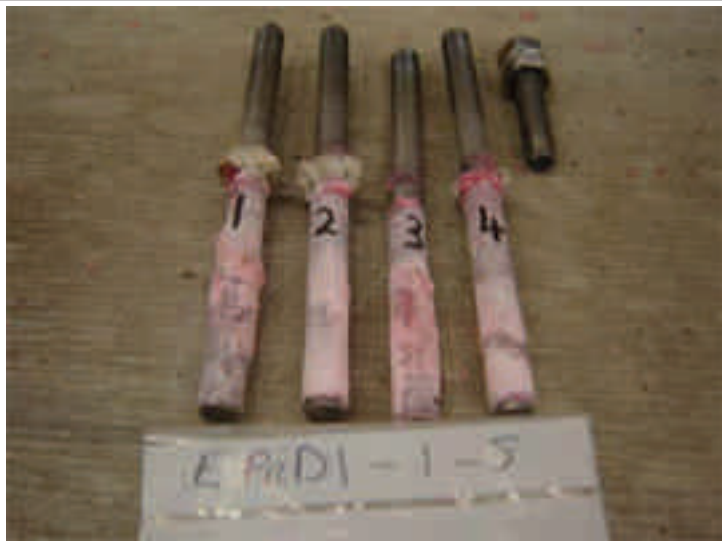
Figure 8.14: - Pull-out failure of Test No. EP20-F1 after tensile loading in wet unclean holes
