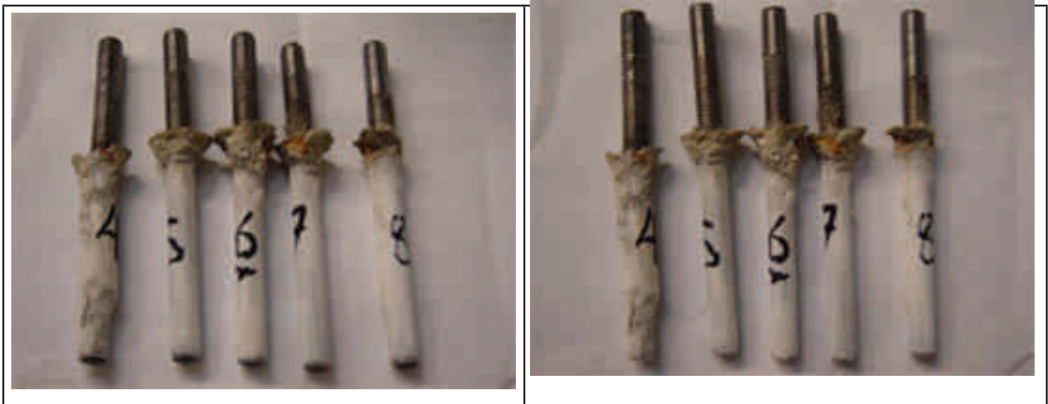
Figure 8.1: - Pull-out failure of Test No. EF8-A1 after tensile loading in dry cleaned hole
