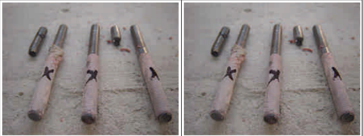
Figure 8.10: - Pull-out failure of Test No. EX8-A1 after tensile loading in dry cleaned holes
