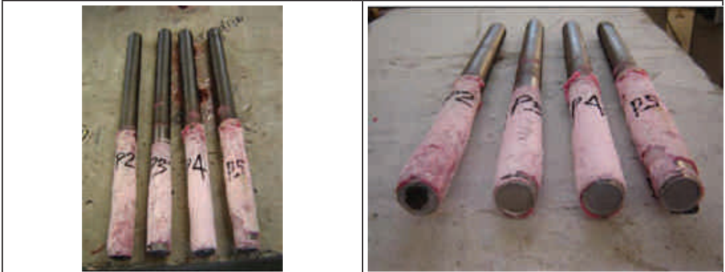
Figure 8.9: - Pull-out failure of Test No. EP20-A1 after tensile loading in dry cleaned holes
