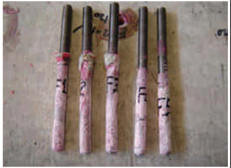
Figure 8.13: Pull-out failure of Test No. EP12-F1 after tensile loading in wet unclean holes
