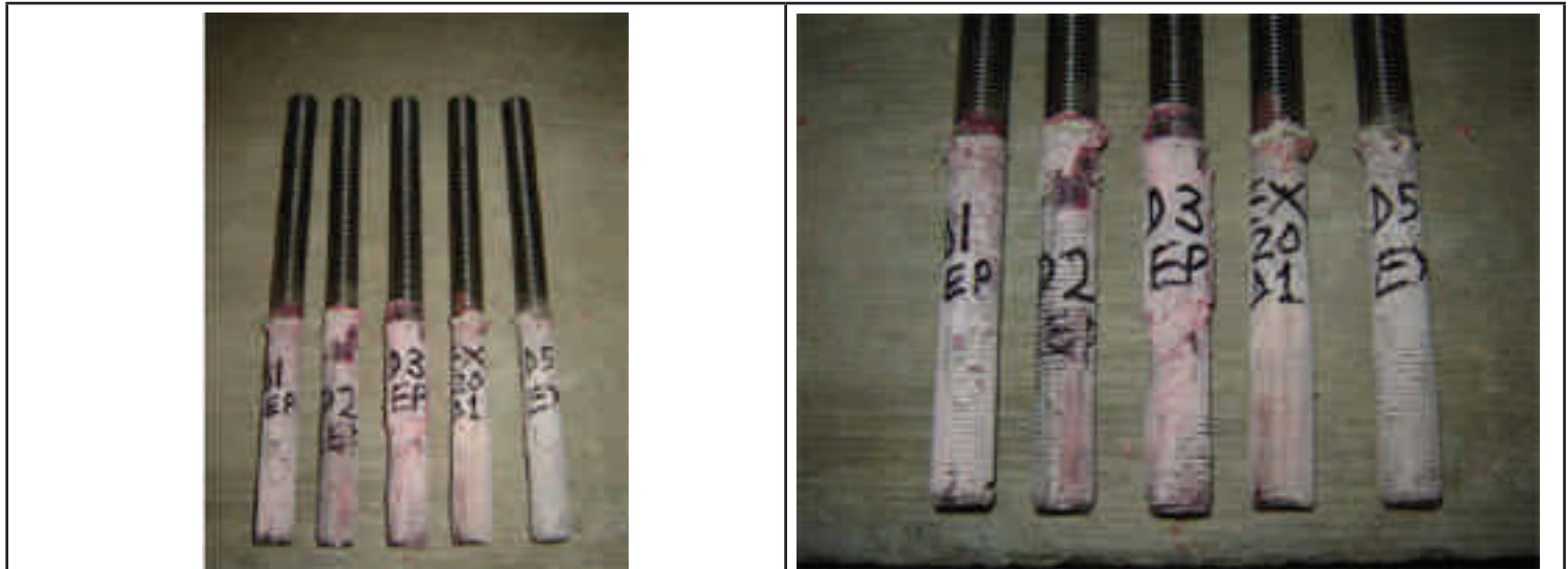
Figure 8.16: - Pull-out failure of Test No. EX20-D1 after tensile loading in diamond drilled holes
