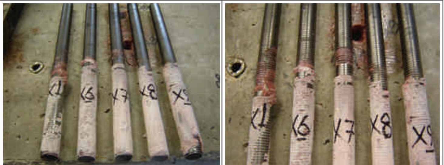
Figure 8.12: - Pull-out failure of Test No. EX20-A1 after tensile loading in dry cleaned holes
