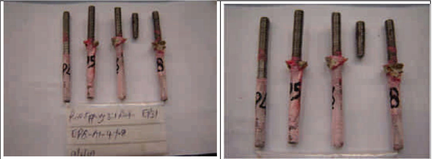
Figure 8.7: - Pull-out failure of Test No. EP8-A1 after tensile loading in dry cleaned holes
