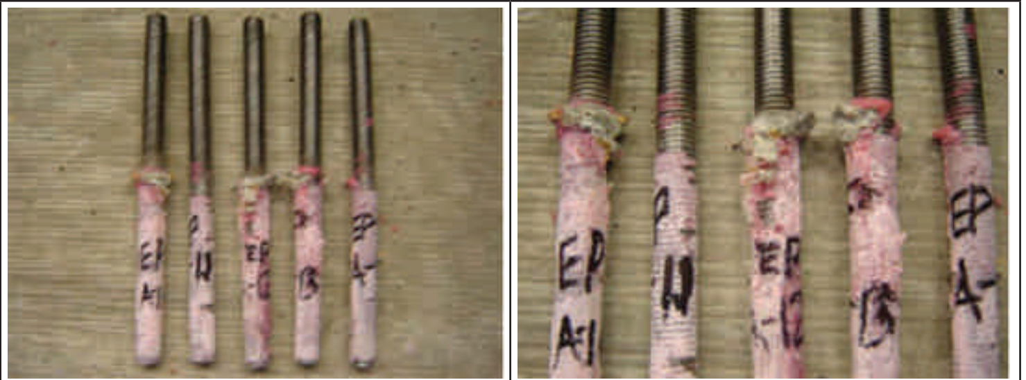
Figure 8.8B: - Pull-out failure of Test No. EP12-A1 after tensile loading in dry cleaned holes – Repeat Tests with 90mm embedment
