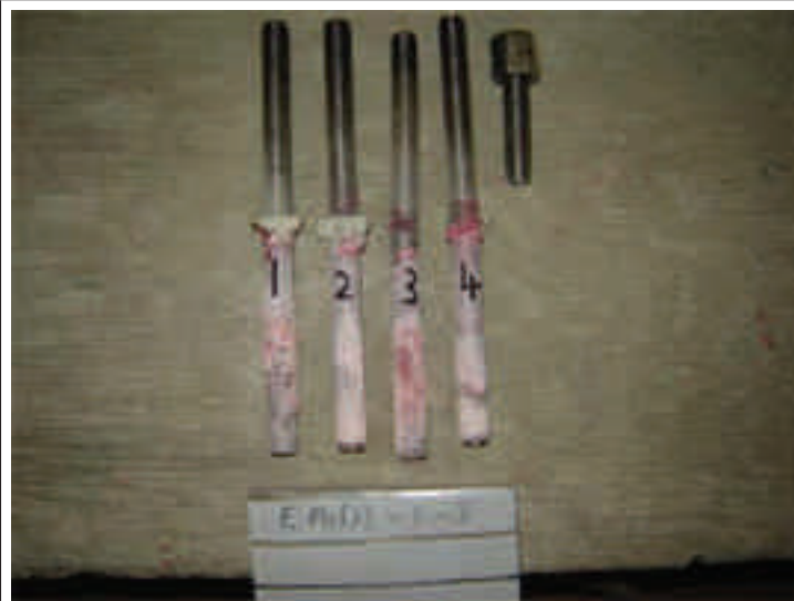
Figure 8.14: - Pull-out failure of Test No. EP20-F1 after tensile loading in wet unclean holes
